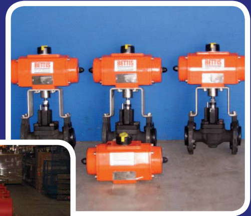
Automated top entry ball valves for a severe service application
